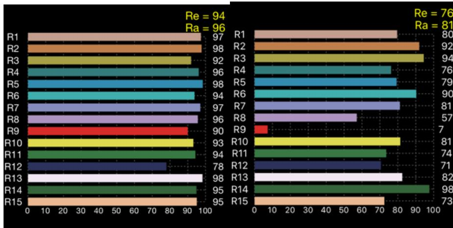
Figure 3 - "R" values for 95 CRI PrimaLine tape light (left) and a competitor's 85 CRI tape light (right).
