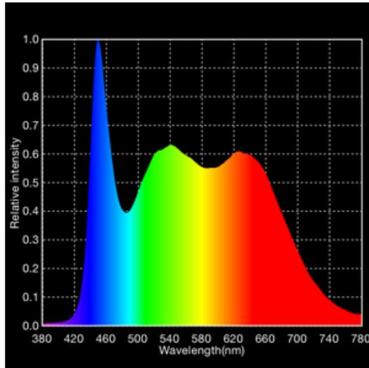
*Figure 2 – 95 CRI PrimaLine tape light spectrograph*
