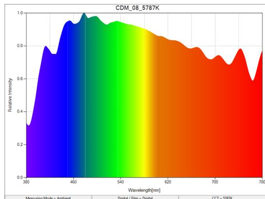
Figure 1 - Spectrograph of daylight
