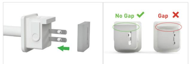
b) Thread the plastic cover onto the PrimaLine Neon Tape Light where the tape light will connect to power. Make sure that the grooves on the inside the plastic cover are aligned with the indentations on the sides of the tape light. (Continued on next page)
