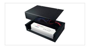
Building codes often require that wire connections be separated into compartments. These junction boxes separate the low voltage and high voltage connections into separate compartments, and are useful for connections between LED fixtures and low voltage power. Each model has a size dedicated to fit specific driver models.
