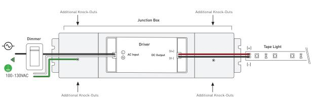
Wiring diagram is for reference ONLY. Please refer to dimmer wiring specifications sheet for accurate directions.
