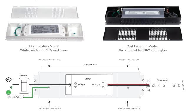
Wiring diagram is for reference ONLY. Please refer to dimmer wiring specifications sheet for accurate directions.
