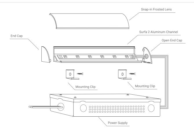
Easily snap lens into mounted channel
