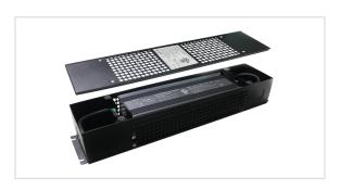
0-10V dimmable LED drivers are designed to integrate into existing 0-10V dimming systems and provide smooth, efficient power and dimming capability for LED lighting. These drivers include an inspection-ready UL Listed junction box enclosure and offer unparalleled performance for 0-10V systems. These drivers are already derated, which means they can be loaded to maximum wattage capacity.
