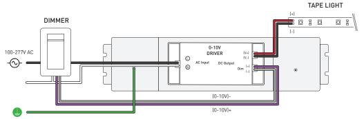
Note: Dimmer switch wiring for reference use only. Please follow wiring instructions provided with the dimmer switch.
