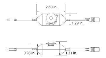
The Inline Rotary Dimmer provides simple dimming and on/off control for LED lights. Featuring male and female DC plugs, this LED dimmer plugs directly into Alloy LED's non-dimmable plug-in adapters and DC accessories. This easy-to-use accessory is compact and great for temporary and low-impact installations.
