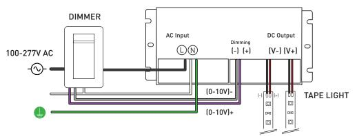
Note: Dimmer switch wiring for reference use only. Please follow wiring instructions provided with the dimmer switch.
