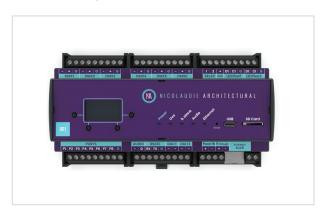
Designed for din-rail mounting, the DR1 is a strong and durable solution for fixed lighting installations. Up to 3072 channels (1024 RGB or 768 RGBW fixtures) can be controlled over several protocols: DMX 512, Art-Net or SACN, LED Pixel, DALI. Multiple controllers can be connected and synchronized for large-scale lighting installation.
