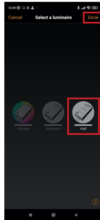
12) Select the luminaire(s) to control and select "Done"
