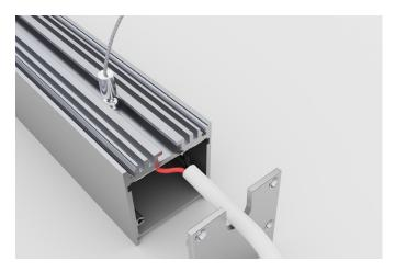
8. First loosen the screw in the channel mount, then slide the mount with screw into the base of the channel, positioning it a few inches from the end of the channel, and tighten using the mount.
