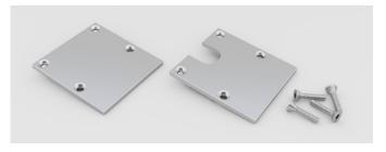
2. Channel end caps are available in both open (left) and closed (right) models. The open notch end cap lets the power wire pass from the inside of the channel to the DC power supply. On the other end of the channel, the closed end cap provides a light tight seal.
