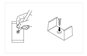
Press one edge of profile into mounting clip.
